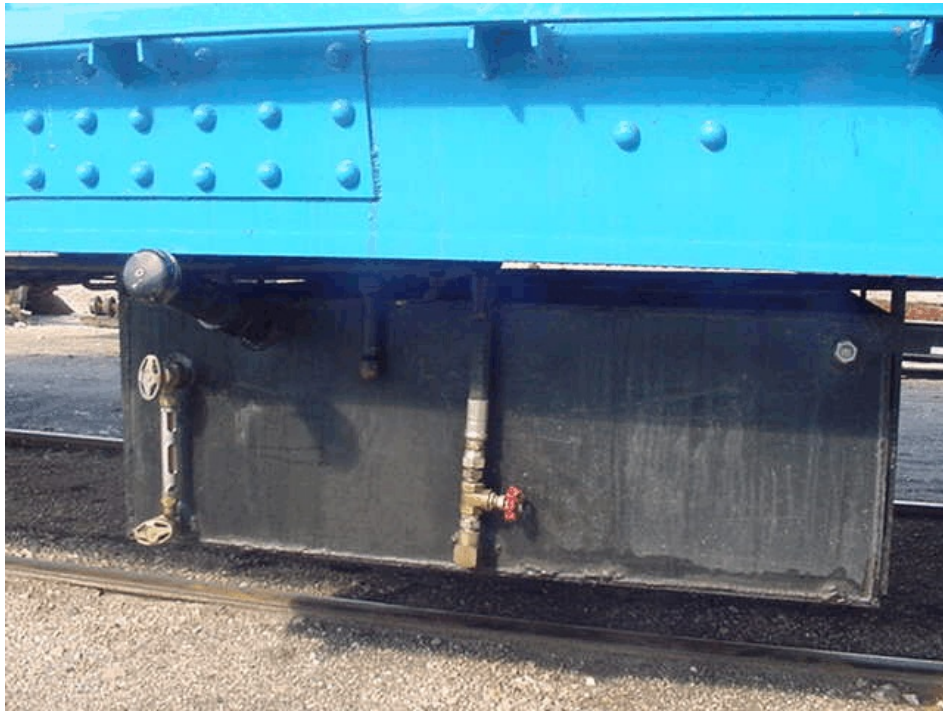
Figure 1. - Fuel Tank Sight Glass
